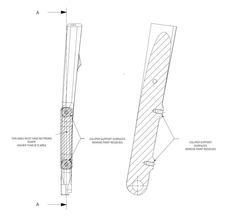
Fig.1 SECTION A - A
