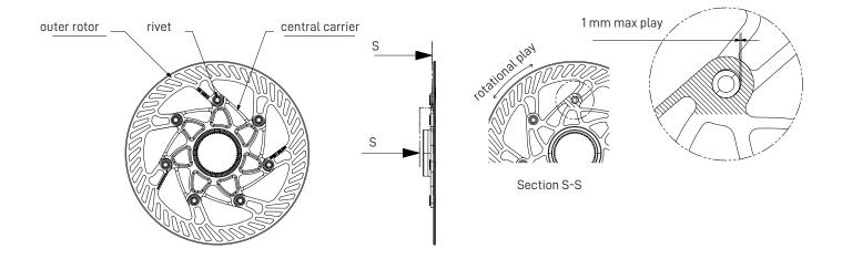
The force that must be used in order to make the play occur may vary significantly between one disc and another, but this a normal consequence of the use of rivets and does not affect the correct operation of the discs themselves.
