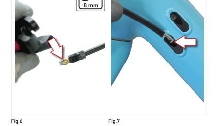
The barb driver on the end of the hose can be used to guide the hose via a rear derailleur hose mounted onto it.
